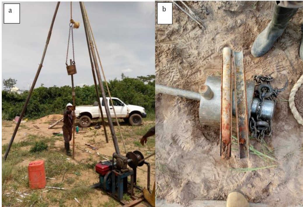
Plate 1: (a)Process of Standard Penetration Test and (b)Recovered spoon sample at the site
